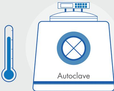
The bag is Autoclaved at 121 °C for 30 minutes (1 cycle)
